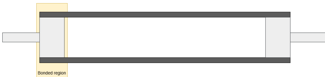
Figure 1. Simplified geometry of a hybrid CFRP-metal roller
