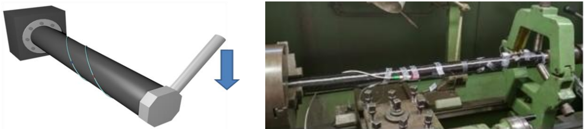
Fig. 2. (a) Torque tests experimental set up for buckling sensor development, (b) Torque experiment
